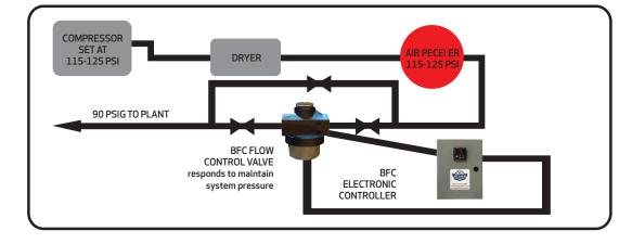
The BFC Flow Control Valve delivers constant air pressure to the plant, reduces compressed air Energy/KW, reduces compressed air Flow/consumption.
